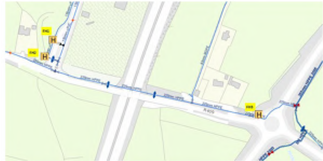
Figure 3-5. Extract from Hydrant Pressure Testing Report – Hydrant Locations and Test Results
